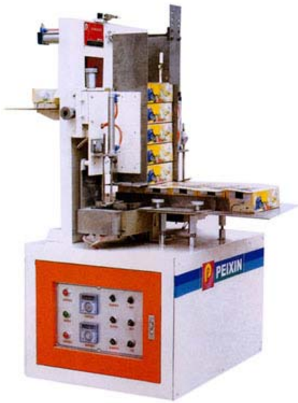
YX-ZFJ-50 Automatic Sealing Cardboard Box Machine
